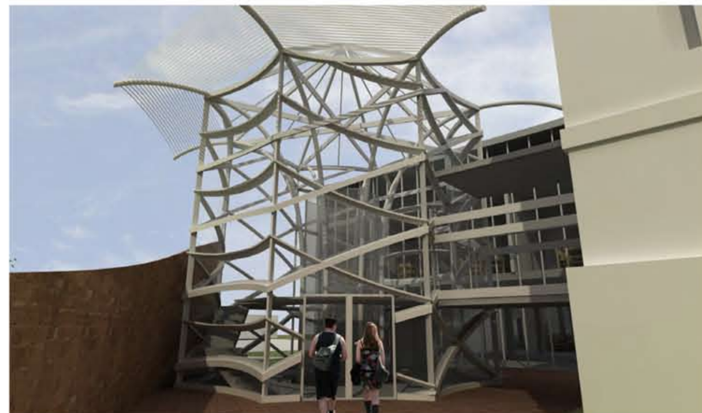
A close-up of the circulation core reveals its airy nature and sculptural quality. Web-like sunshades extend to the south to shade the structure. The core is portal through which pedestrians enter the addition from the existing library. It acts as the counter-point to Richardson's heavy masonry octagon in the existing structure.
