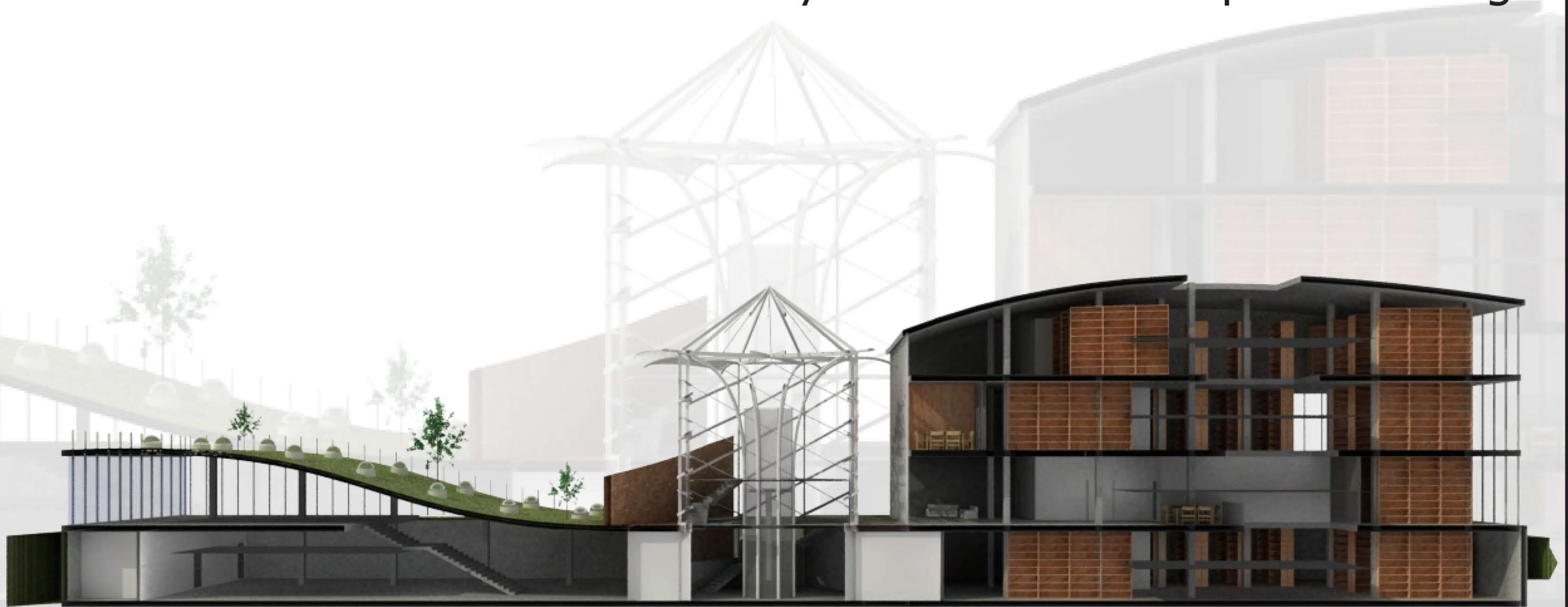
A section through the addition reveals the undulating form and open nature of the space. The two-story community space is separated from the four-story area which houses the stacks by the sculptural circulation core. An open air atrium penetrates down all four stories of the stacks to take advantages of daylight penetration.
